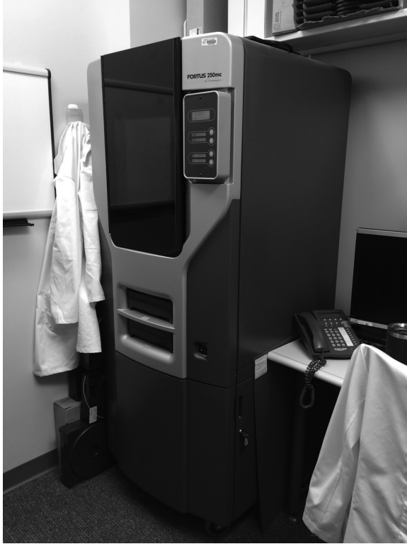
Fig. 3 In-office Fortus 250 3D printer. (Reprinted with permission from Adam Schwartz, MD.)
