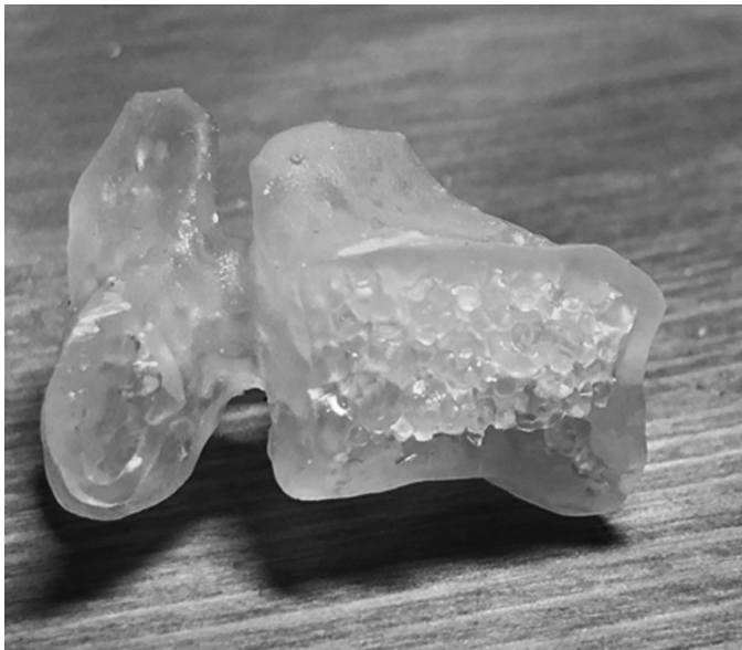
Fig. 2 Section cut of 3D-printed vertebrae showing internal mesh trabecular structure while housed within a thick cortical wall. Model was printed with 100% clear resin off the Form 2 SLA printer. (Reprinted with permission from John Hao, PhD.)
